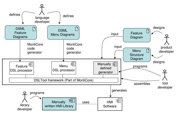
Figure 2: Generator structure for the HMI
