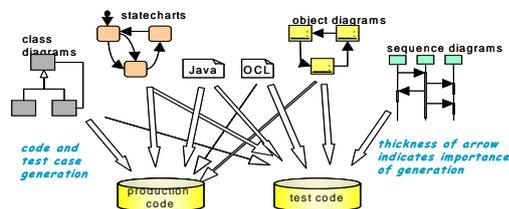
**Fig. 1.** Mapping of UML-models to code and test code Some of the UML-models (mainly deployment and class diagrams as well as statecharts) are used constructively, while others are used for test case definition (mainly OCL, sequence and enhanced object diagrams). The following Fig. 1 illustrates the key mappings from various diagrams to the
